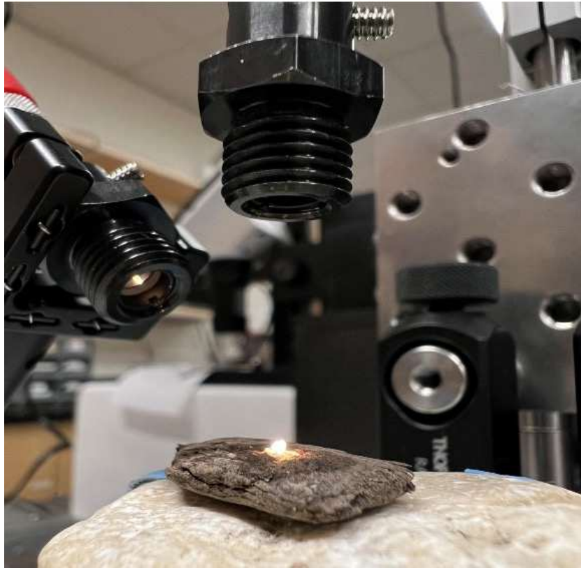
Figure SI 1 The photograph depicts a plastic sample being measured while placed on a piece of bark that has been wetted with water. Photo by K.A.R.
