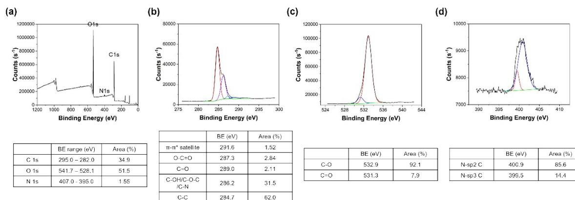
**Figure S15.** XPS spectra collected for KL-PhBZ-A: (a) survey spectrum; (b) C region with fits for C-C sp<sup>2</sup> and sp<sup>3</sup> (red), C-OH/C-O-C/C-N (purple), O=C=O (light blue), C=O (blue),  $\pi$ - $\pi^*$  satellites (pink); (c) O region with fits for C=O (blue), C-OH/C-O-C (red); (d) N region with fits for N-sp<sup>2</sup> C (red) and N-sp<sup>3</sup> C (blue). The background is shown in green. The tables underneath each graph summarise the results from fitting the data.
