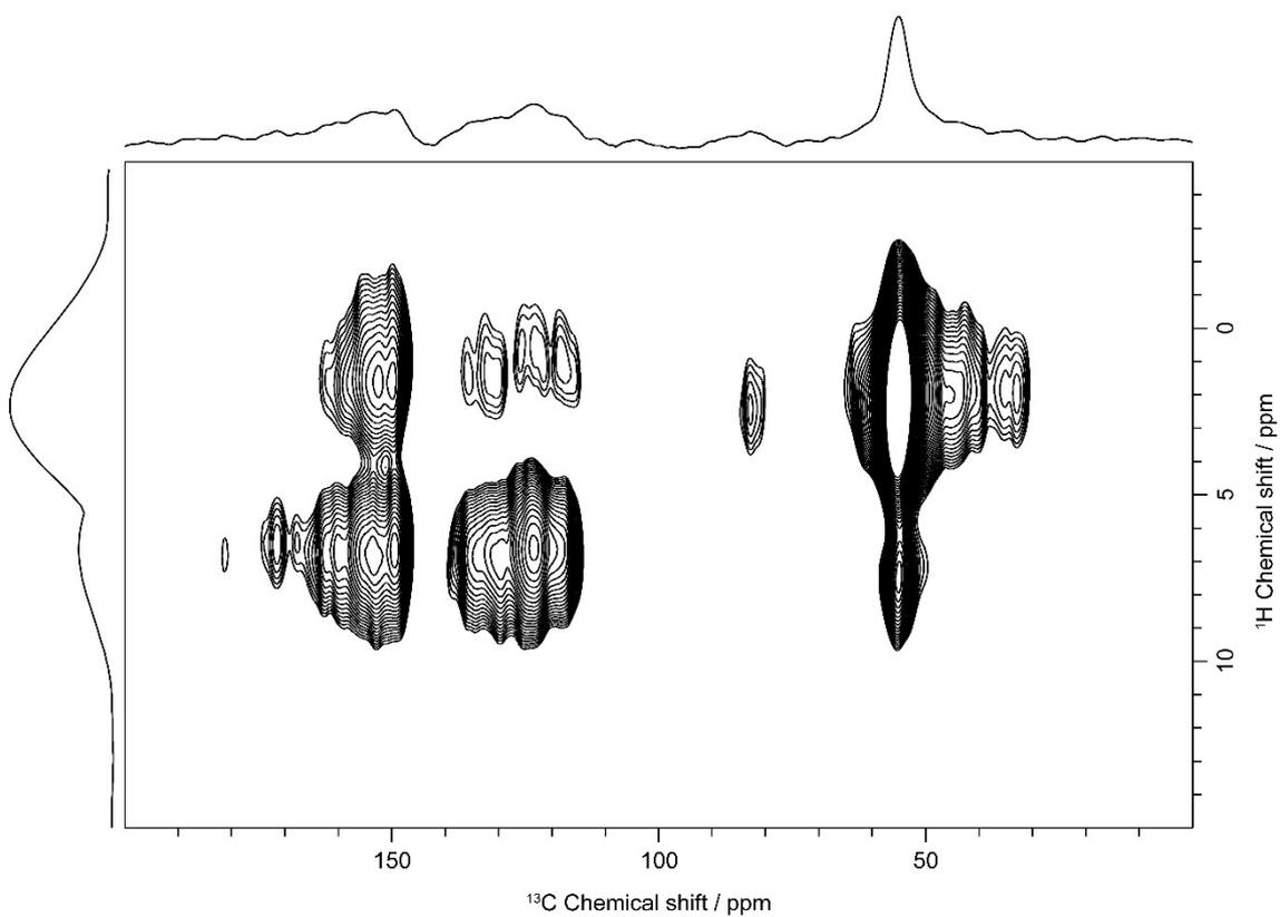
**Figure S21:** 2D  $^1\text{H}$ - $^{13}\text{C}$  HETCOR NMR spectrum of SL-BZ-B lignin, measured with a cross polarisation contact time of 1 ms.
