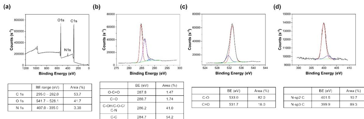
**Figure S7.** XPS spectra collected for KL-BZ-A: (a) survey spectrum; (b) C region with fits for C-C sp<sup>2</sup> and sp<sup>3</sup> (red), C-OH/C-O-C/C-N (purple), O-C=O (light blue), C=O (blue); (c) O region with fits for C=O (blue), C-OH/C-O-C (red); (d) N region with fits for N-sp<sup>2</sup> C (red) and N-sp<sup>3</sup> C (blue). The background is shown in green. The tables underneath each graph summarise the results from fitting the data.
