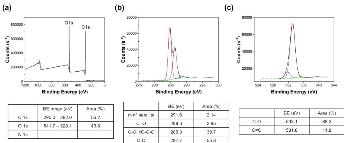
**Figure S5.** XPS spectra collected for KL: (a) survey spectrum; (b) C region with fits for C-C sp2 and sp3 (red), C-OH/C-O-C/C-N (purple), C=O (blue),  $\pi$ - $\pi^*$  satellites (pink); (c) O region with fits for C=O (blue) and C-OH/C-O-C (red). The background is shown in green. The tables underneath each graph summarise the results from fitting the data.
