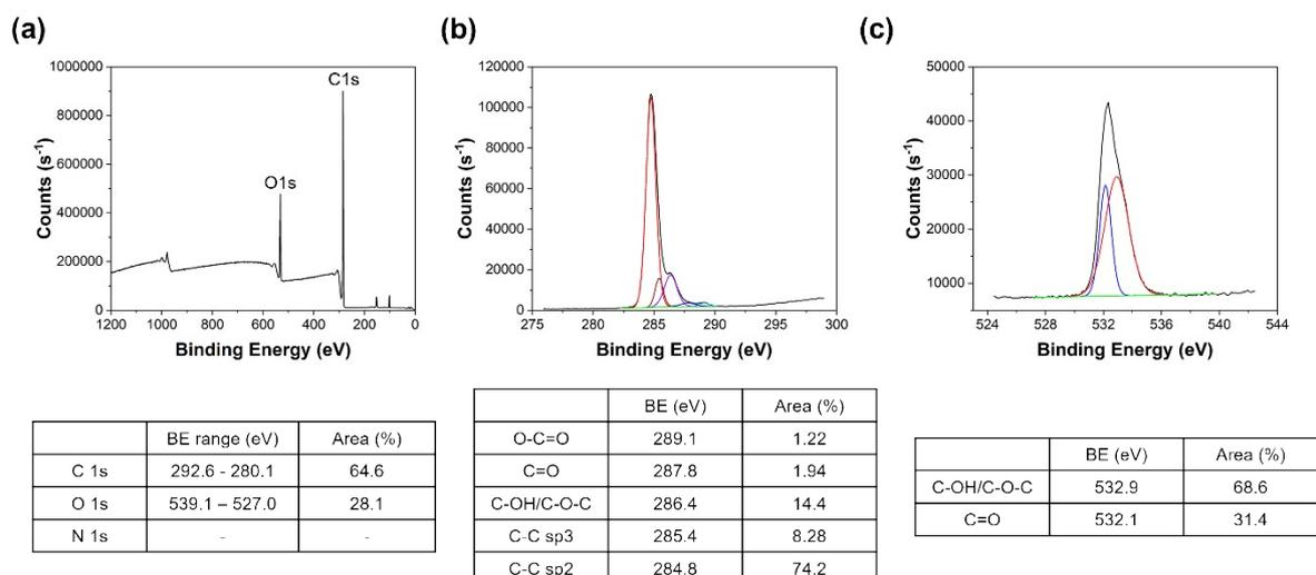
**Figure S1.** XPS spectra collected for unmodified Sonichem lignin: (a) survey spectrum; (b) C region with fits for C-C sp<sup>2</sup> (red), C-C sp<sup>3</sup> (dark red), C-OH/C-O-C (purple), O-C=O (light blue), C=O (blue); (c) O region with fits for C=O (blue) and C-OH/C-O-C (red). The background is
