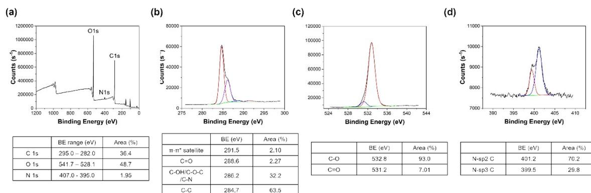
**Figure S14.** XPS spectra collected for KL-PhBZ-aniline: (a) survey spectrum; (b) C region with fits for C-C sp<sup>2</sup> and sp<sup>3</sup> (red), C-OH/C-O-C/C-N (purple), C=O (blue),  $\pi$ - $\pi^*$  satellites (pink); (c) O region with fits for C=O (blue), C-OH/C-O-C (red); (d) N region with fits for N-sp<sup>2</sup> C (red) and N-sp<sup>3</sup> C (blue). The background is shown in green. The tables underneath each graph summarise the results from fitting the data.
