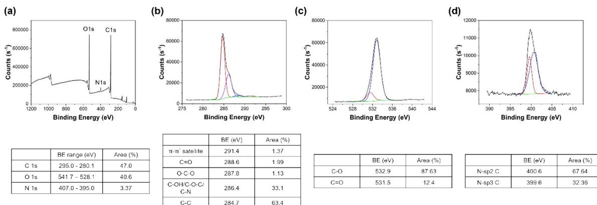
**Figure S10.** XPS spectra collected for SL-PhBZ-aniline: (a) survey spectrum; (b) C region with fits for C-C sp2 (red), C-C sp3 (dark red), C-OH/C-O-C/C-N (purple), O-C=O (light blue), C=O (blue),  $\pi$ - $\pi^*$  satellites (pink); (c) O region with fits for C=O (blue), C-OH/C-O-C (red); (d) N
