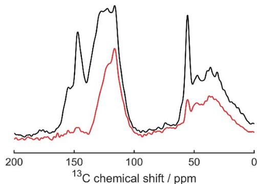
**Figure S18.**  $^{13}\text{C}$  CP MAS NMR spectra of Kraft lignin, functionalised with phenol and/or benzoxazine, detected with a CP contact time of 1 ms (black) and 50  $\mu\text{s}$  (red).
