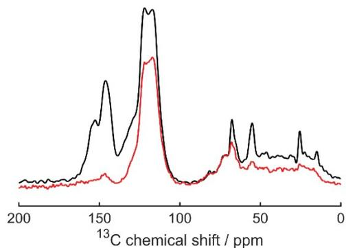
**Figure S17.**  $^{13}\text{C}$  CP MAS NMR spectra of Sonichem lignin, functionalised with phenol and/or benzoxazine, detected with a CP contact time of 1 ms (black) and 50  $\mu\text{s}$  (red).
