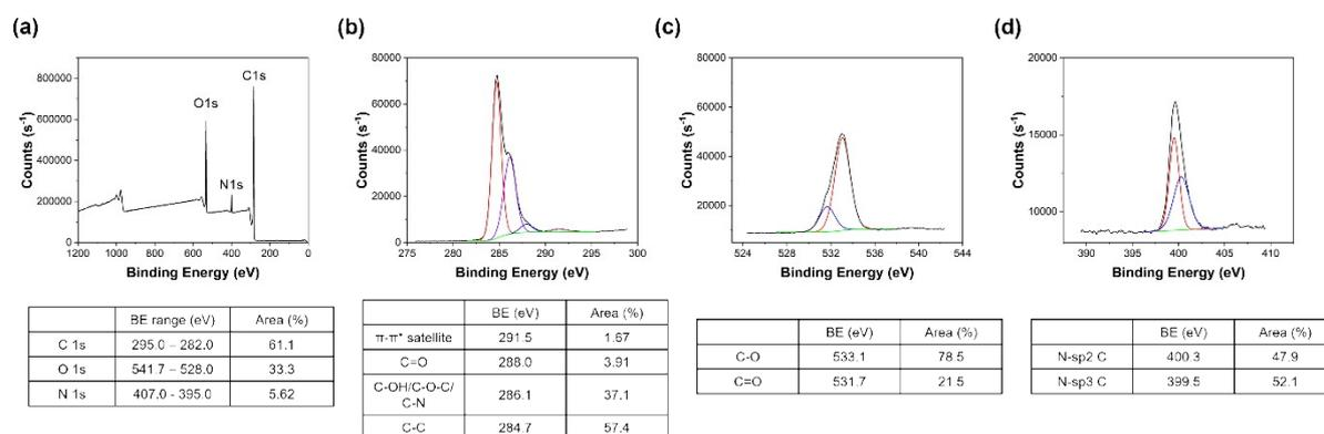
**Figure S6.** XPS spectra collected for KL-BZ-aniline: (a) survey spectrum; (b) C region with fits for C-C sp<sup>2</sup> and sp<sup>3</sup> (red), C-OH/C-O-C/C-N (purple), C=O (blue),  $\pi$ - $\pi^*$  satellites (pink); (c) O region with fits for C=O (blue), C-OH/C-O-C (red); (d) N region with fits for N-sp<sup>2</sup> C (red) and N-sp<sup>3</sup> C (blue). The background is shown in green. The tables underneath each graph summarise the results from fitting the data.
