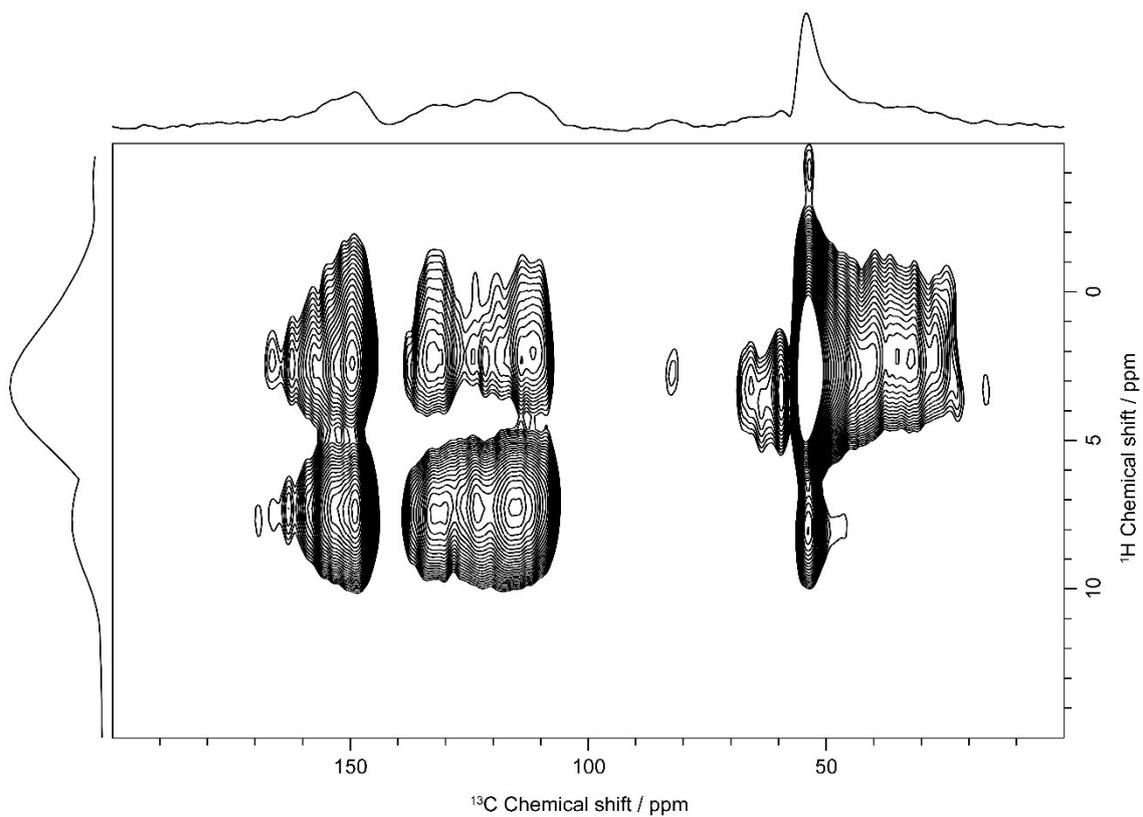
**Figure S19:** 2D  $^1\text{H}$ - $^{13}\text{C}$  HETCOR NMR spectrum of SL lignin, measured with a cross polarisation contact time of 1 ms.
