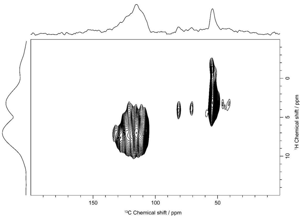
**Figure S20:** 2D  $^1\text{H}$ - $^{13}\text{C}$  HETCOR NMR spectrum of SL lignin, measured with a cross polarisation contact time of 50  $\mu\text{s}$ .
