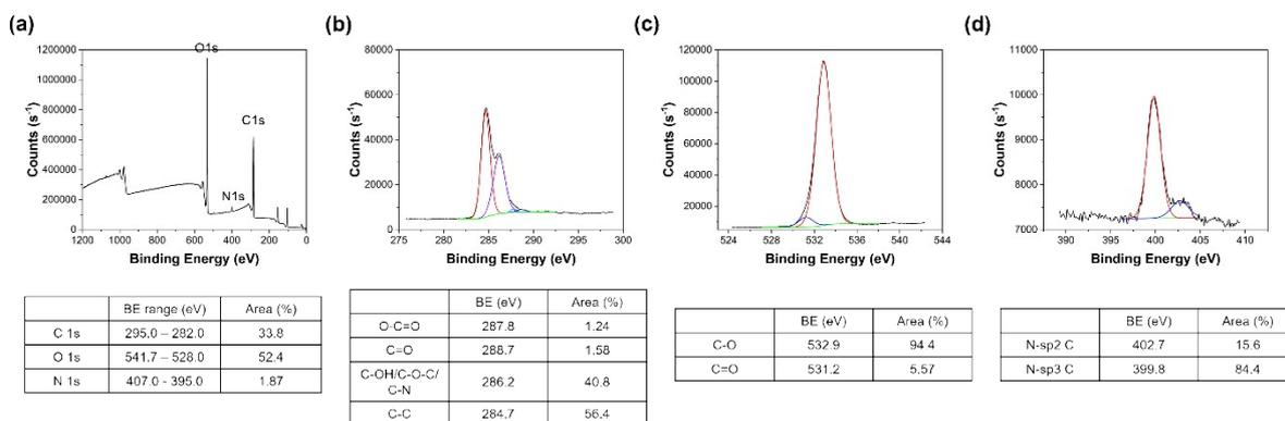
**Figure S8.** XPS spectra collected for KL-BZ-B: (a) survey spectrum; (b) C region with fits for C-C sp2 and sp3 (red), C-OH/C-O-C/C-N (purple), O-C=O (light blue), C=O (blue); (c) O region with fits for C=O (blue), C-OH/C-O-C (red); (d) N region with fits for N-sp2 C (red) and N-sp3 C (blue). The background is shown in green. The tables underneath each graph summarise
