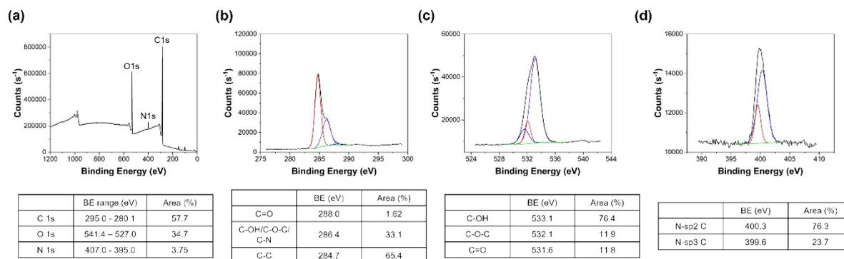
**Figure S11.** XPS spectra collected for SL-PhBZ-A: (a) survey spectrum; (b) C region with fits for C-C sp<sup>2</sup> and sp<sup>3</sup> (red), C-OH/C-O-C/C-N (purple), C=O (blue); (c) O region with fits for C=O (blue), C-OH (purple) and C-O-C (red); (d) N region with fits for N-sp<sup>2</sup> C (red) and N-sp<sup>3</sup> C (blue). The tables underneath each graph summarise the results from fitting the data.
