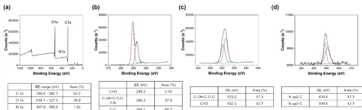
**Figure S12.** XPS spectra collected for SL-PhBZ-B: (a) survey spectrum; (b) C region with fits for C-C sp<sup>2</sup> and sp<sup>3</sup> (red), C-OH/C-O-C/C-N (purple), C=O (blue); (c) O region with fits for C=O (blue), C-O (red); (d) N region with fits for N-sp<sup>2</sup> C (red) and N-sp<sup>3</sup> C (blue). The background is shown in green. The tables underneath each graph summarise the results from fitting the data.
