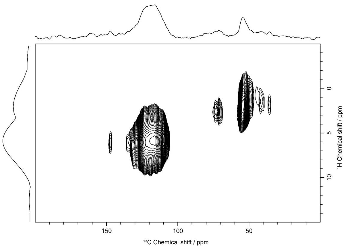
**Figure S22:** 2D  $^1\text{H}$ - $^{13}\text{C}$  HETCOR NMR spectrum of SL-BZ-B lignin, measured with a cross polarisation contact time of 50  $\mu\text{s}$ .
