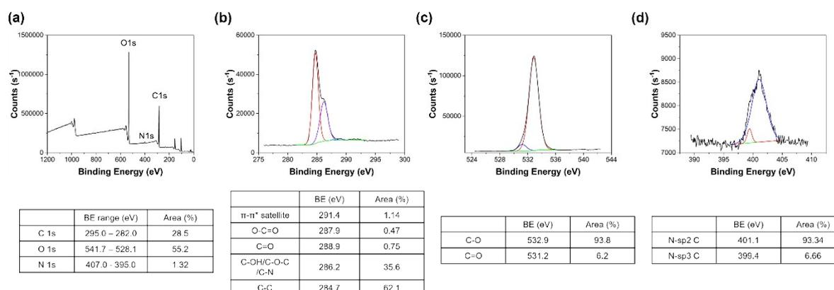
**Figure S16.** XPS spectra collected for KL-PhBZ-B: (a) survey spectrum; (b) C region with fits for C-C sp<sup>2</sup> and sp<sup>3</sup> (red), C-OH/C-O-C/C-N (purple), O=C=O (light blue), C=O (blue),  $\pi$ - $\pi^*$  satellites (pink); (c) O region with fits for C=O (blue), C-OH/C-O-C (red); (d) N region with fits for N-sp<sup>2</sup> C (red) and N-sp<sup>3</sup> C (blue). The background is shown in green. The tables underneath each graph summarise the results from fitting the data.
