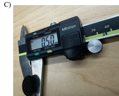
Figure S2. A) CAD model of the designed anode (I) Isometric view, (II) front view (diameter), and (III) side view (thickness), B) pictures of the (I) as-printed sample, and (II) pyrolyzed sample, C) the measured thickness of the as-printed sample, and D) the measured thickness of the pyrolyzed sample.
