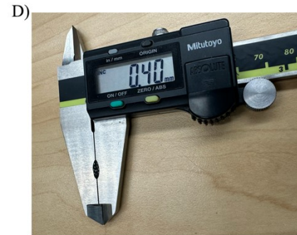
Figure S2. A) CAD model of the designed anode (I) Isometric view, (II) front view (diameter), and (III) side view (thickness), B) pictures of the (I) as-printed sample, and (II) pyrolyzed sample, C) the measured thickness of the as-printed sample, and D) the measured thickness of the pyrolyzed sample.
