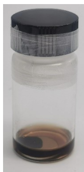
Fig. S13. Image of discharged FQ/rGO films immersed in DMC for 30 days
