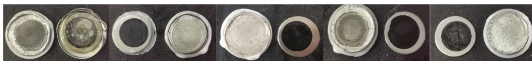
Fig. S12. The pictures of randomly selected and disassembled cells after long cycle tests
