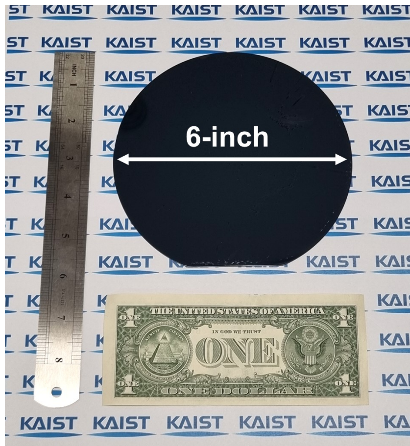
Figure S3. Fabricated BCP on a 6-inch Si wafer. By using BCP self-assembly, nanopatterns could be fabricated in wafer-scale.
