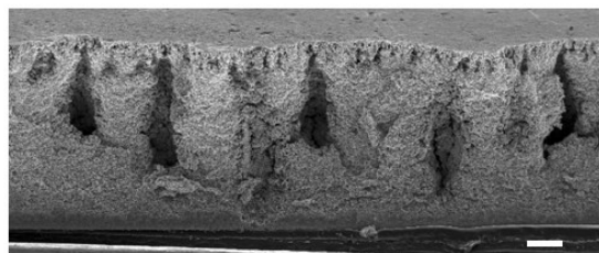
Fig. S15. SEM images of (a) WE31-20 and (b) WE31-30 electrodes (scale bar: 100 \mu\text{m} ).
