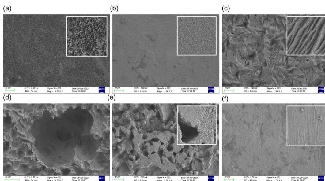
**Figure S2.** SEM morphology obtained after etching with different etchants (a)-(f) 5% NaOH, 5% HNO<sub>3</sub>, 5% HCl, 5% H<sub>2</sub>SO<sub>4</sub>, 5% H<sub>2</sub>C<sub>2</sub>O<sub>4</sub>, Bare Zn. Scale bar is 10 μm and the top right zoom is 1 μm.
