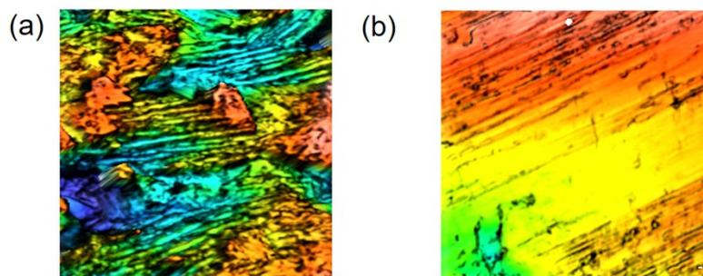
**Figure S3.** Comparison of profilometer maps of Zigzag Zn(a) and bare Zn(b).
