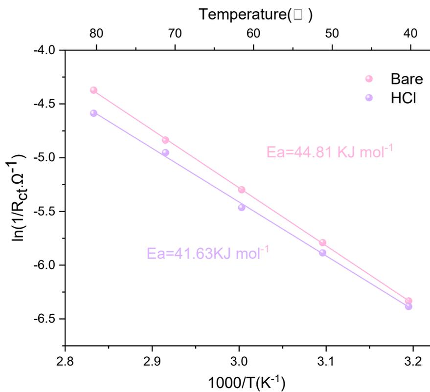
**Figure S12.** Arrhenius curves and activation energy of zinc ion diffusion.
