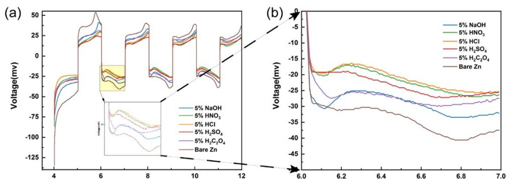
**Figure S7.** Polarization curves of symmetric cells using different etching reagents at the current density of  $1 \text{ mA cm}^{-2}$  and areal capacity of  $1 \text{ mAh cm}^{-2}$  and the (b) zoomed-in partial view.
