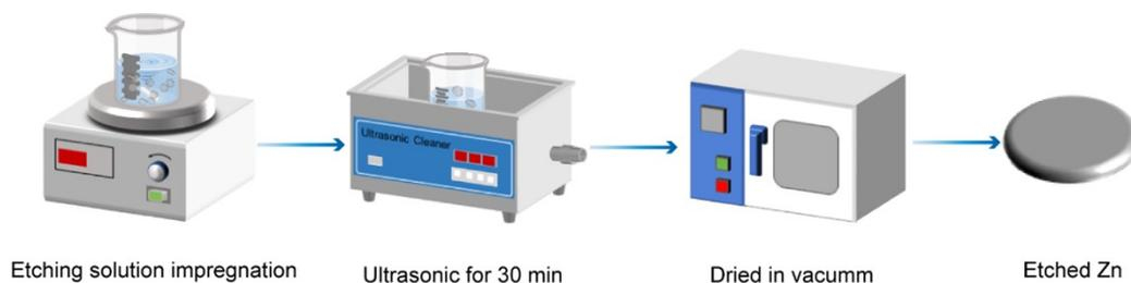
**Figure S1.** Preparation flow chart of zigzag Zn anode.
