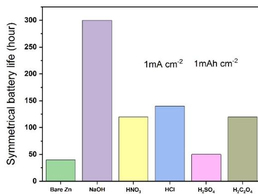
**Figure S5.** Cycle life of different symmetric cells.
