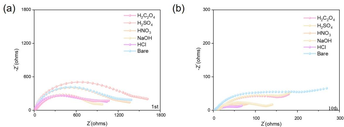
**Figure S6.** Comparisons of EIS spectra for bare, HCl, NaOH,  $HNO_3$ ,  $H_2SO_4$ ,  $H_2C_2O_4$  Zn batteries after the 1<sup>st</sup> (a) and 10<sup>th</sup> (b) cycles in aqueous  $Zn(OTf)_2$  electrolyte.
