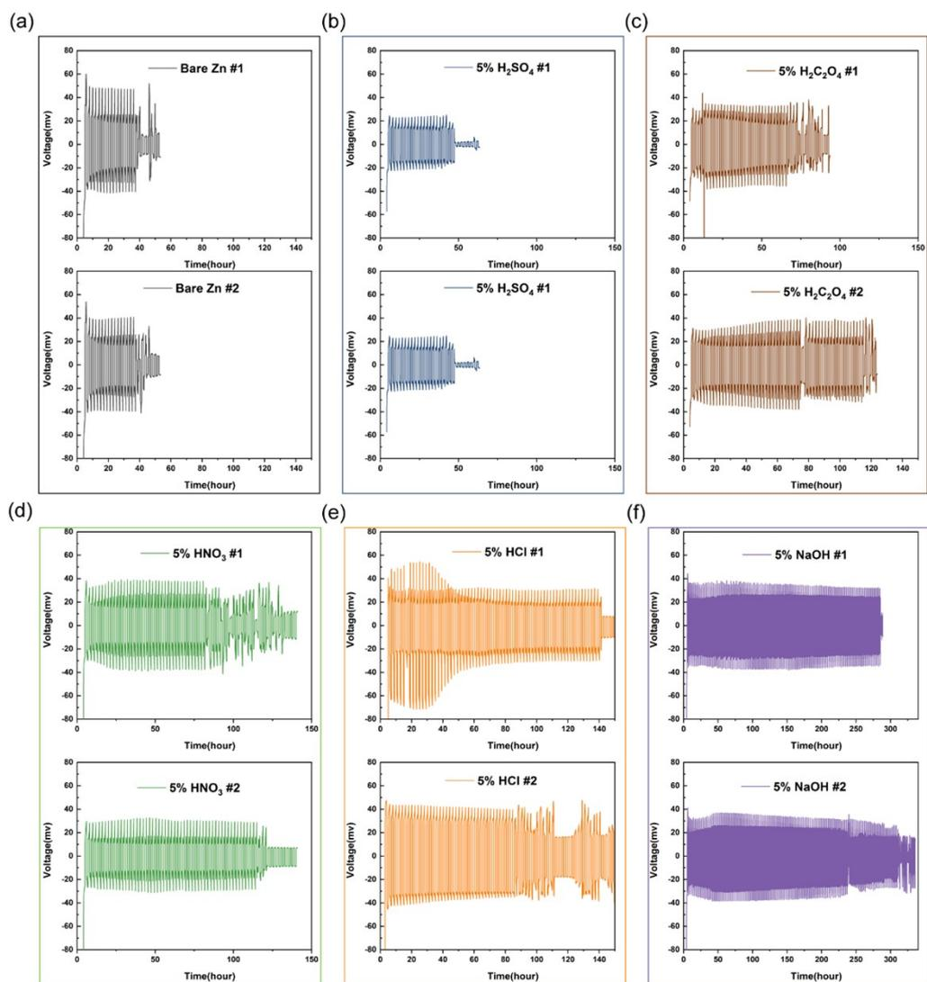
**Figure S4.** Cycling performance of symmetric cells assembled from Zn foil after etching with different reagents.
