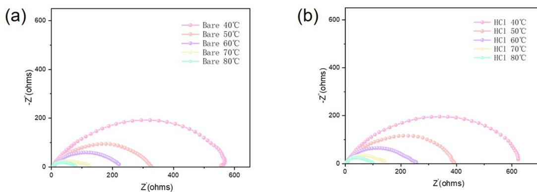
**Figure S11.** Nyquist plots of Zn//Zn cells at different temperatures in (a) bare Zn and (b) Zigzag Zn.
