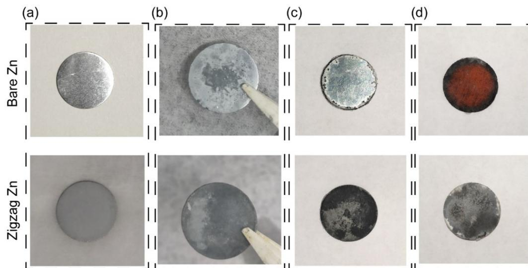
**Figure S10.** (a) Photograph of bare Zn and zigzag Zn after HCl etching and (b) Zn electrode in symmetric cell after 30 cycles under  $1 \text{ mA cm}^{-2}$ . (c) Photograph of the Zn electrode of Zn-Cu half-cell after 30 cycles of  $1 \text{ mA cm}^{-2}$  and (d) the corresponding Cu electrodes.
