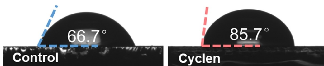
Figure S9. Water contact angles of the control and Cyclen films.
