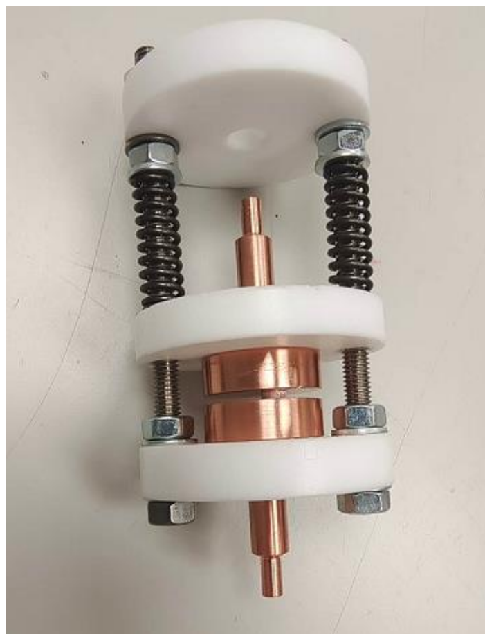
Figure S1. Digital photograph of the pellet sample testing cell with two plate electrodes.
