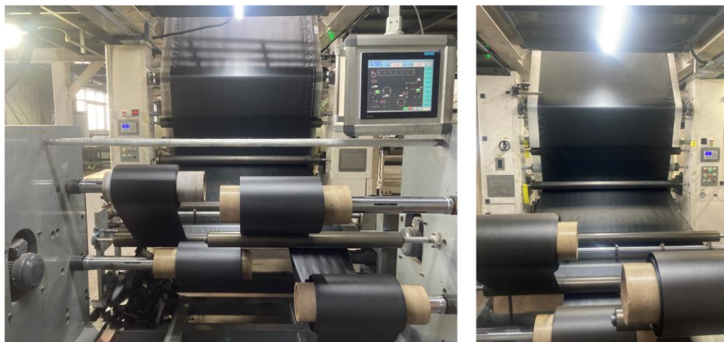
Fig. S1 Digital photos of industrialized coated preparation of graphene oxide films.
