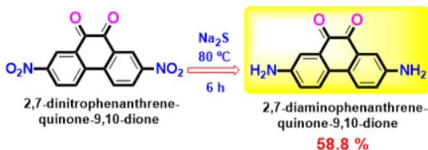
Scheme S2: Schematic representation for the synthesis of 2,7-diaminophenanthrenequinone-9,10-dione.
