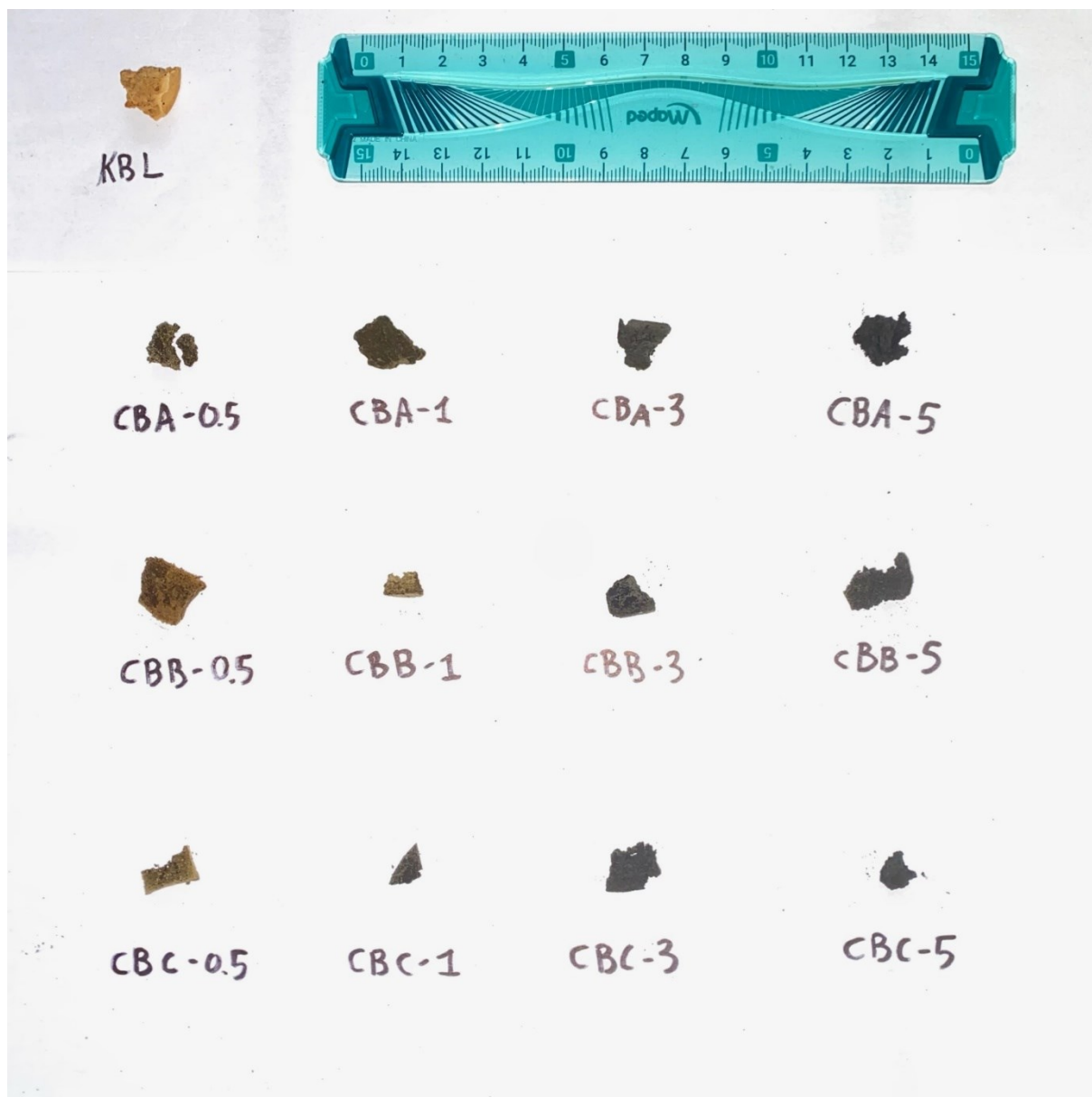
Figure S7: Photography of obtained monolith blocks of the different synthesized samples synthesized. The blocks presented here are cut from their respective samples after the drying step. Ruler in centimetre for scale.
