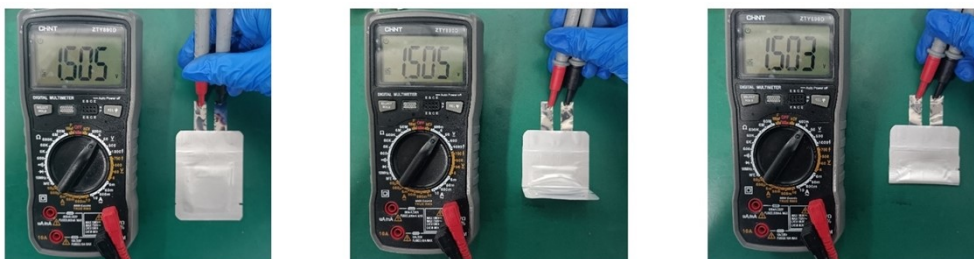
Fig. S31. The effect of different levels of folding on the voltage of pouch cells. Demonstrating the potential for flexible electronics applications.
