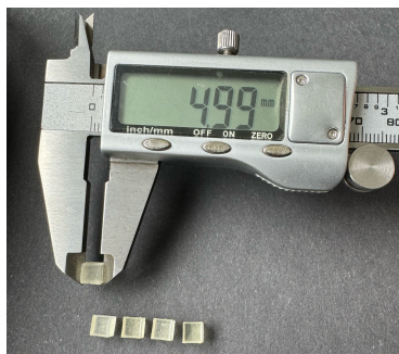
Fig. S8. Photo of 3D printed RIH3 5x5x5 mm cubes, showcasing dimensional stability
