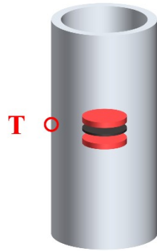
Figure S2. Schematic diagram of the thermocouple location in a vacuum tube high-temperature sintering furnace.
