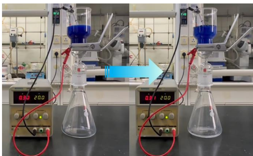
Figure S17. The catalytic reaction of MB aqueous solution with 0.1 M \text{Na}_2\text{SO}_4 was realized by applying voltage switch to change the wettability of Pd/ZIF-8@CC-DCA membrane.
