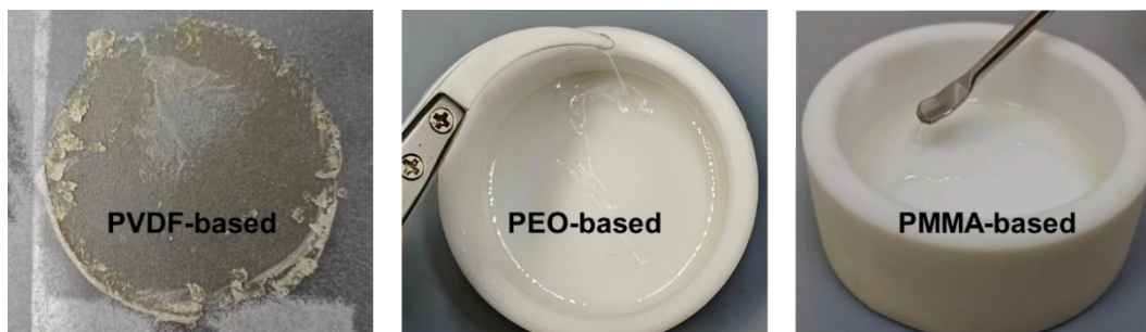
Fig. S3 Digital photographs of 10 wt%PVDF/90 wt%CSE gel, 10 wt% PEO/90 wt%CSE gel, and 10 wt%PMMA/90 wt%CSE gel.
