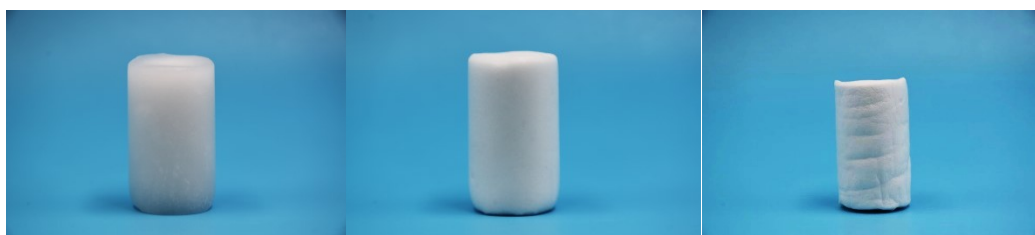
Figure S3. The photos of unpigmented spongy-like hydrogel, wet sponge and dried sponge.
