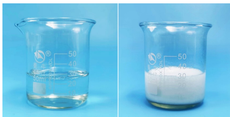
Figure S2 The change of PVA/glycerol/CaCl 2 solution from transparent to milk-white state with the addition of Na 3 Cit.
