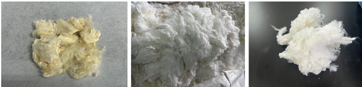
Fig. S4. The photograph of the alginic (left), cellulose (middle), and low melt polylactic acid/polylactic acid bicomponent fibers (right).
