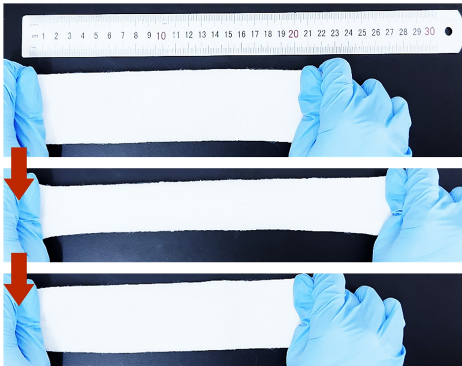
Fig. S12. The photograph of the ensile elastic behaviour of the prepared samples of laminated elastic fabric named MR-FL 40.3.
