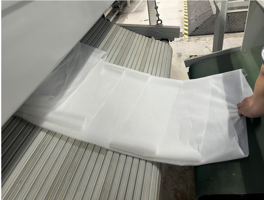
Fig. S3. The photograph of the PBE filaments webs after the cross-lapping process.
