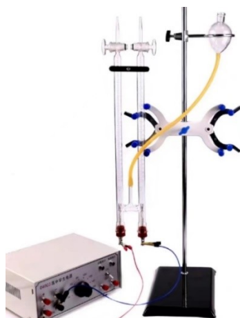
Fig. S40 The Hoffmann electrolytic device for overall water splitting.
