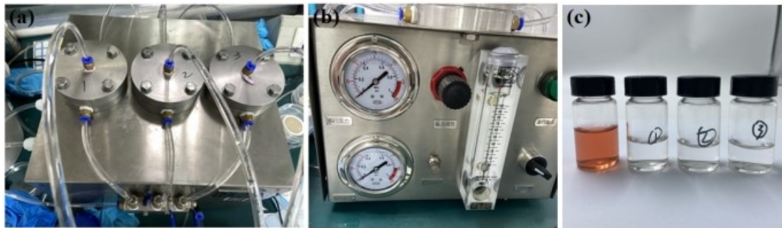
Fig. S3 (a-b) Top view and main view of cross-flow filtration apparatus, (c) Mother liquid and permeate liquid before and after separation of the M4 membrane.
