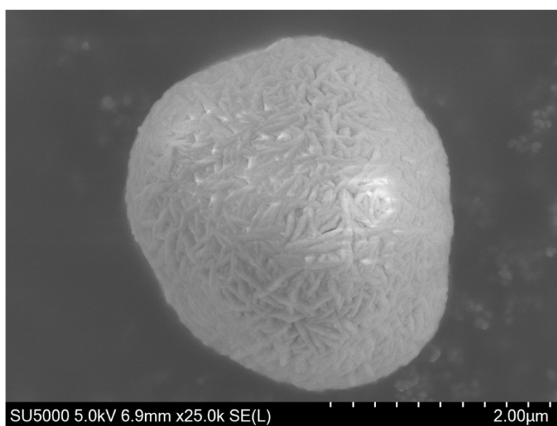
Fig. S12† SEM image of \text{Ni}_{0.96}\text{Co}_{0.02}\text{Mn}_{0.02}(\text{OH})_2 precursor
