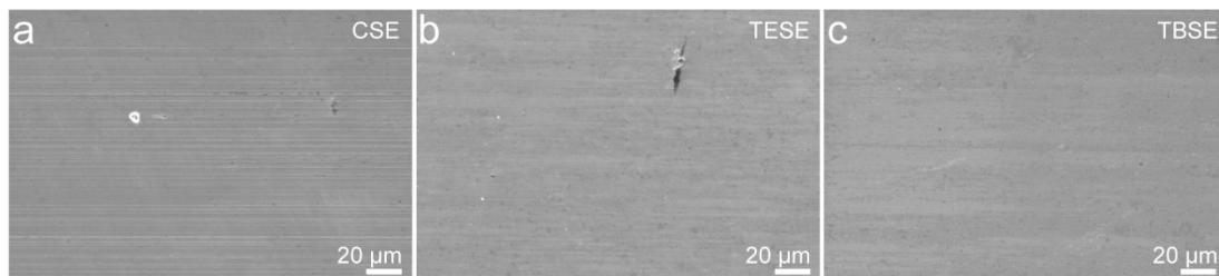
Fig. S14 Anti-wear performance. SEM images of wear tracks lubricated by (a) CSE, (b) TESE and (c) TBSE TDESs under high relative humidities (80% RH).
