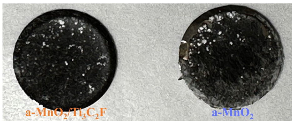
Figure S14. Photographs of a-MnO 2 /Ti 3 C 2 F and a-MnO 2 cathodes after 500 cycles under a current density of 0.3 A g -1 .
