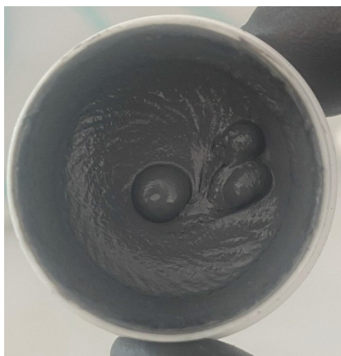
Fig. S-2. Mixed solution of \text{Fe}_{0.5}\text{Mn}_{0.5}\text{O} , \text{NH}_4\text{H}_2\text{PO}_4 , and \text{H}_2\text{O} . The high viscosity indicates \text{Mn}^{2+} dissolution has caused byproducts to form that inherently affect the solution rheology.
