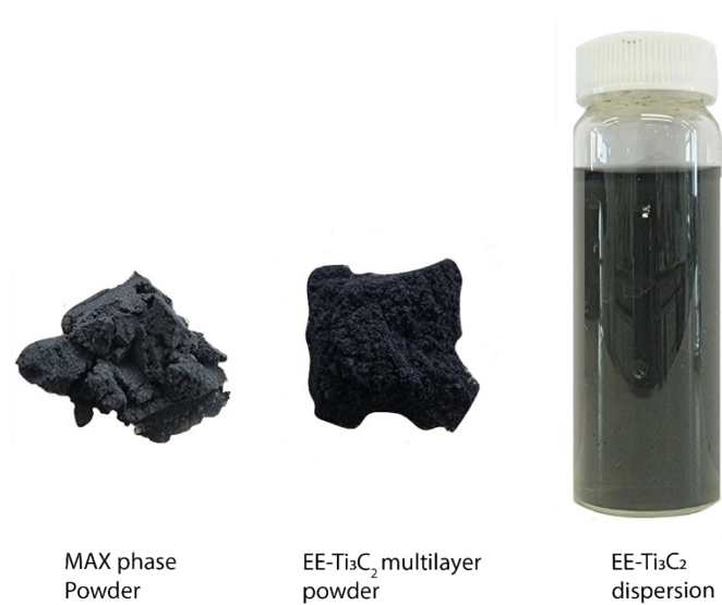
Figure S6. Photographs of Ti_3AlC_2 precursor, EE-Ti_3C_2 multilayer powder, dispersion of TMAOH treated EE-Ti_3C_2 in water.
