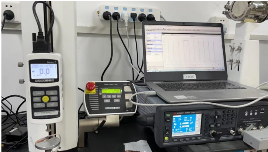
Fig. S5. Photograph of testing platform for evaluating the sensing performance of the flex-occlusometer, comprising a mechanical triggering platform and an electrical signal monitoring system.
