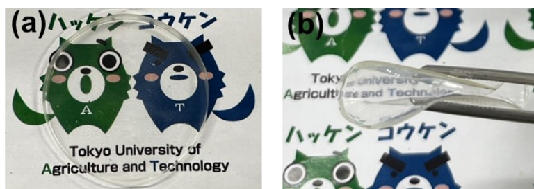
Figure S5 Photographs of CP 29 . (a) CP 29 ( \phi = 35 mm). (b) CP 29 in a bending state.
