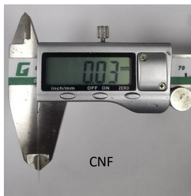
Fig. S3. Digital images of CNF membrane and CNF/GA membrane measured with vernier calipers.
