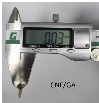
Fig. S3. Digital images of CNF membrane and CNF/GA membrane measured with vernier calipers.
