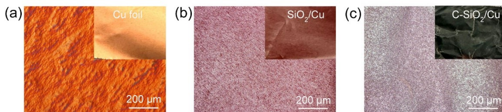
Fig. S2. (a-c) Optical microscopy images: (a) Cu-foil surface (inset digital image), (b) surface of SiO 2 particles deposited on Cu foil (inset digital image), and (c) carbon incorporated SiO 2 particles deposited on Cu foil (inset digital image). A significant surface color changes after deposition of SiO 2 and carbon.
