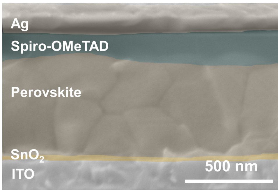
Figure S7. Cross-sectional SEM image of the PSC device based on SnO 2 ETL.
