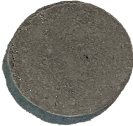
Fig. S1 The pressed pellet sample (the diameter of 12 mm) of Ni/Li 3 N/Mo 2 Ga 2 C with KCl-LiCl molten salts.
