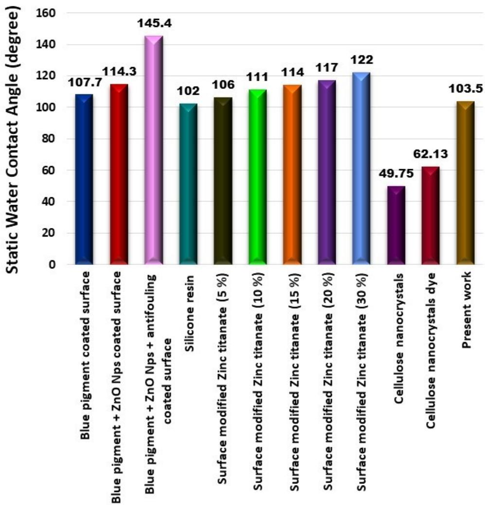
Fig.S6. Comparison of WCA of various pigment coatings with prepared LWFO pigment.
