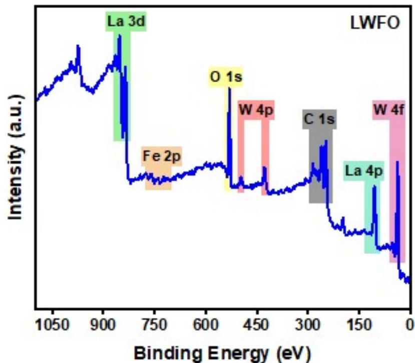
Fig.S2. XPS survey spectrum of the LWFO cooling nano pigment.
