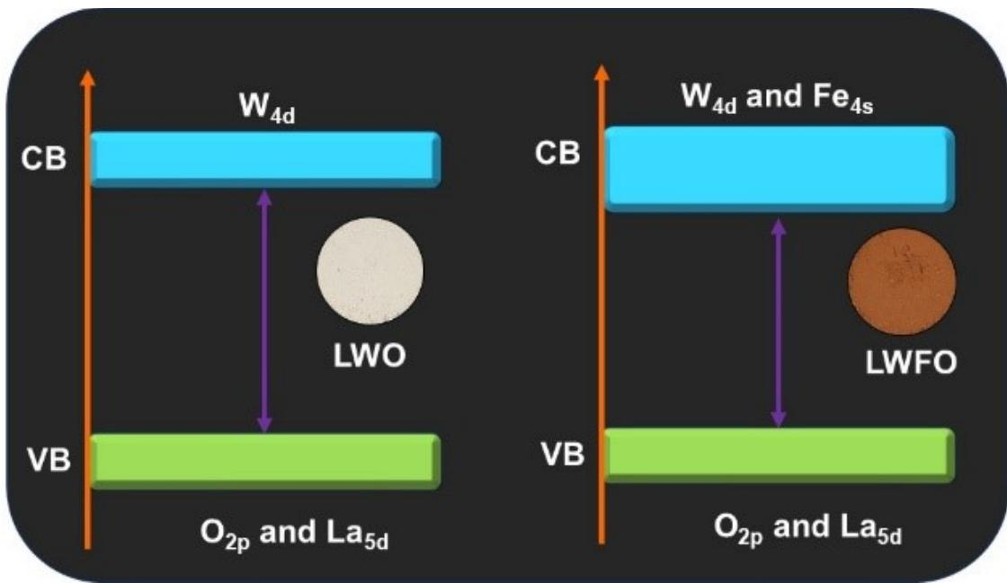
Fig.S4. Schematic illustration demonstrating band structures of LWO and LWFO pigments.
