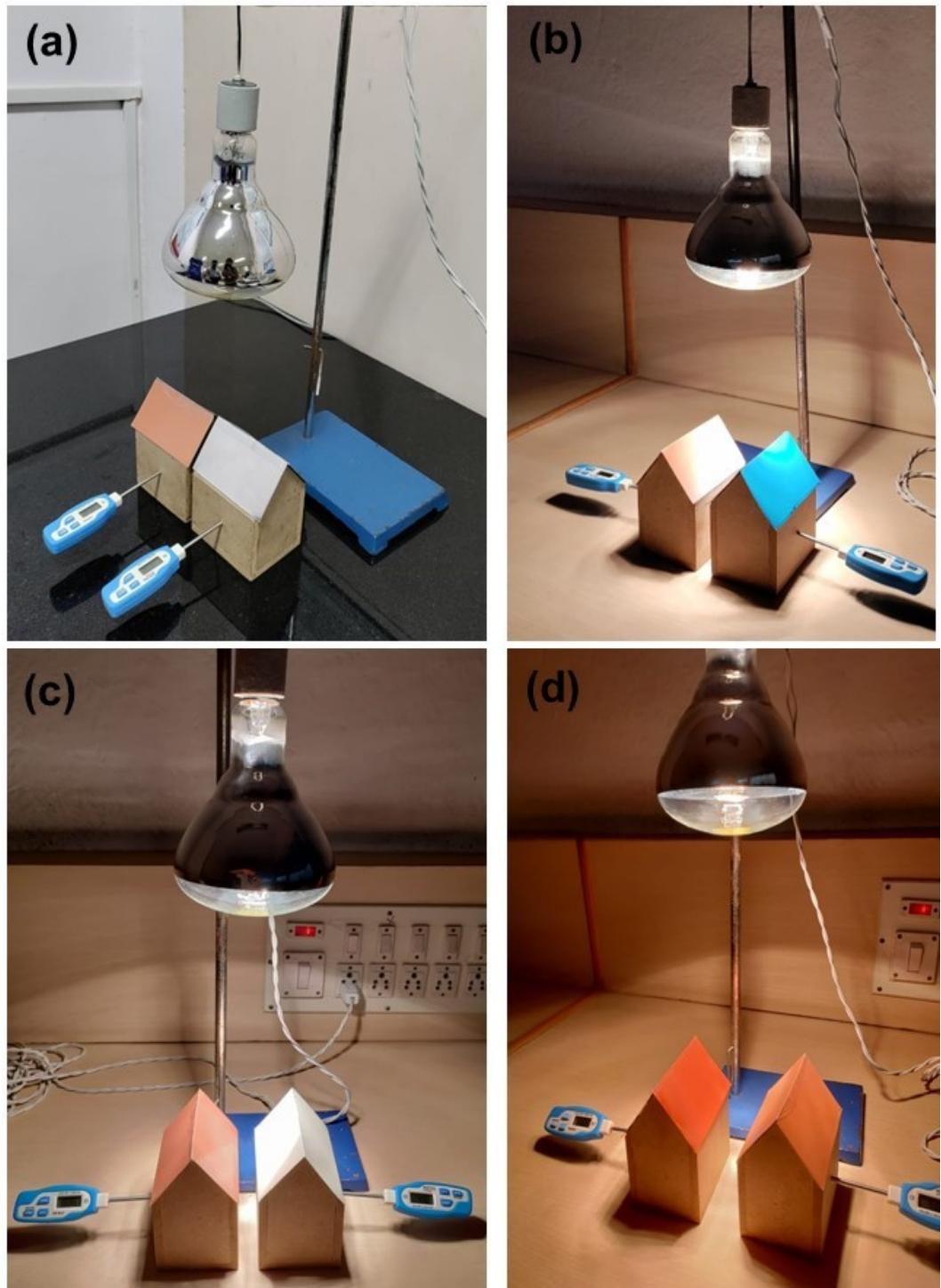
Fig.S5. Photographic images of the house models with different commercially available roofing materials to study passive daytime radiative cooling applications.
