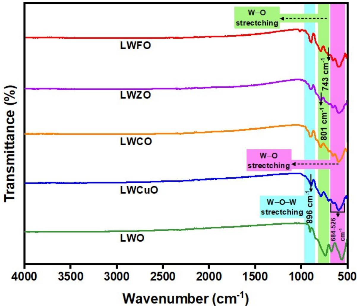
Fig.S3. FTIR spectra of the synthesized cooling nano pigments.
