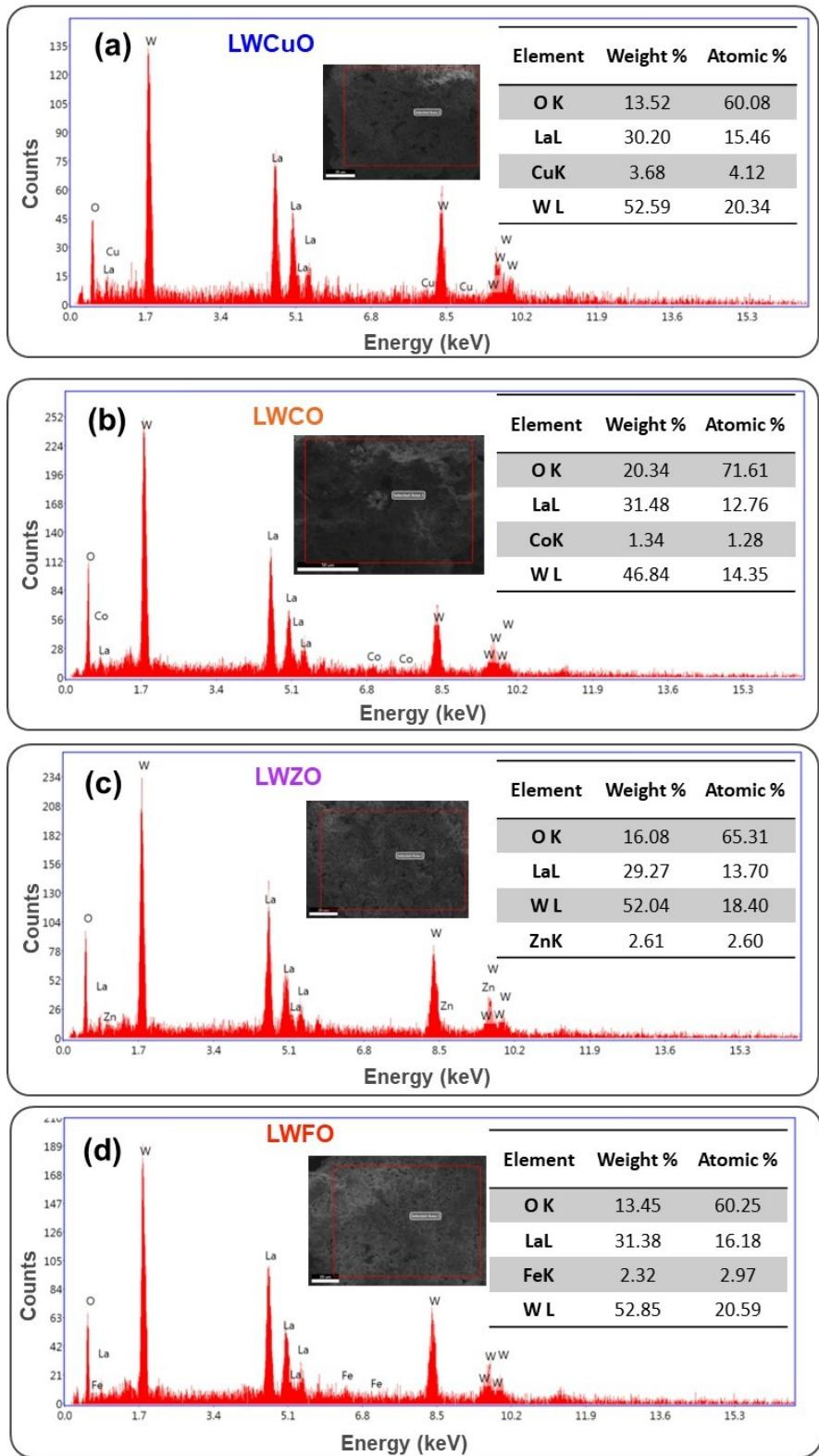
Fig.S1. EDX spectrum of the selected portions of the synthesized LWCuO, LWCO, LWZO, and LWFO nano pigments [Inset: The tables enclosed corresponding elemental compositions in both weight and atomic (in %)].
