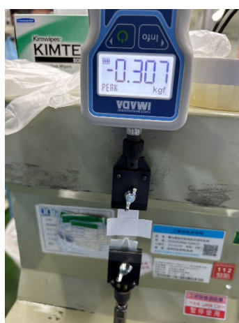
Figure S5. Maximum tensile stress measurement of the polymer electrolyte film.
