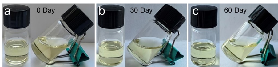
Fig. S2 Optical diagram of stability of DEE-1:4 solutions at room temperature.
