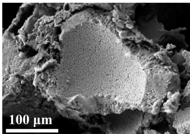
Fig. S2 SEM images of PDMS/GNP<sub>s0.24</sub>@LM<sub>22.1</sub> foam.
