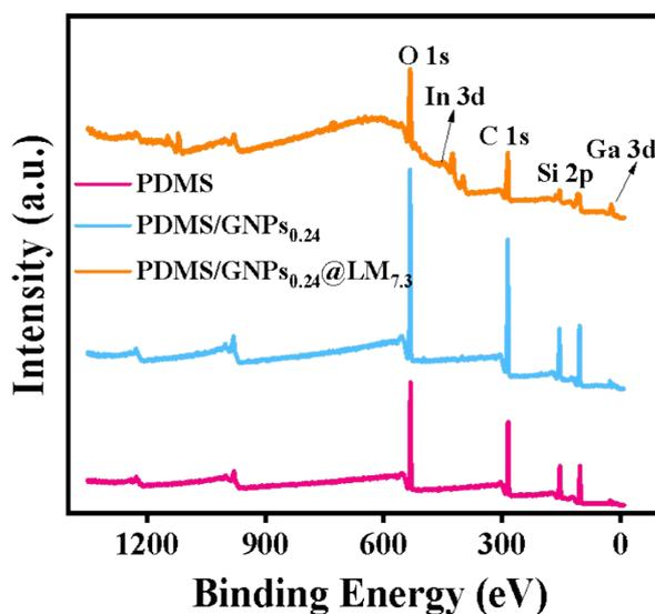
Fig. S1 XPS spectra of neat PDMS, PDMSGNP<sub>s0.24</sub>, and PDMS/GNP<sub>s0.24</sub>@LM<sub>22.1</sub> foam.
