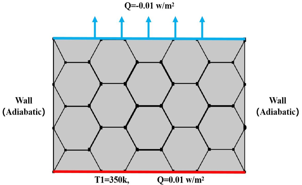
**Fig. S3** Schematic of the boundary conditions for the simulation model.
