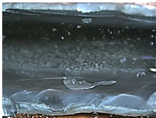
Fig. S3. Schematic of the electrochemical deposition of EDF electrolyte at 100th second in 50 mA cm -2 .
