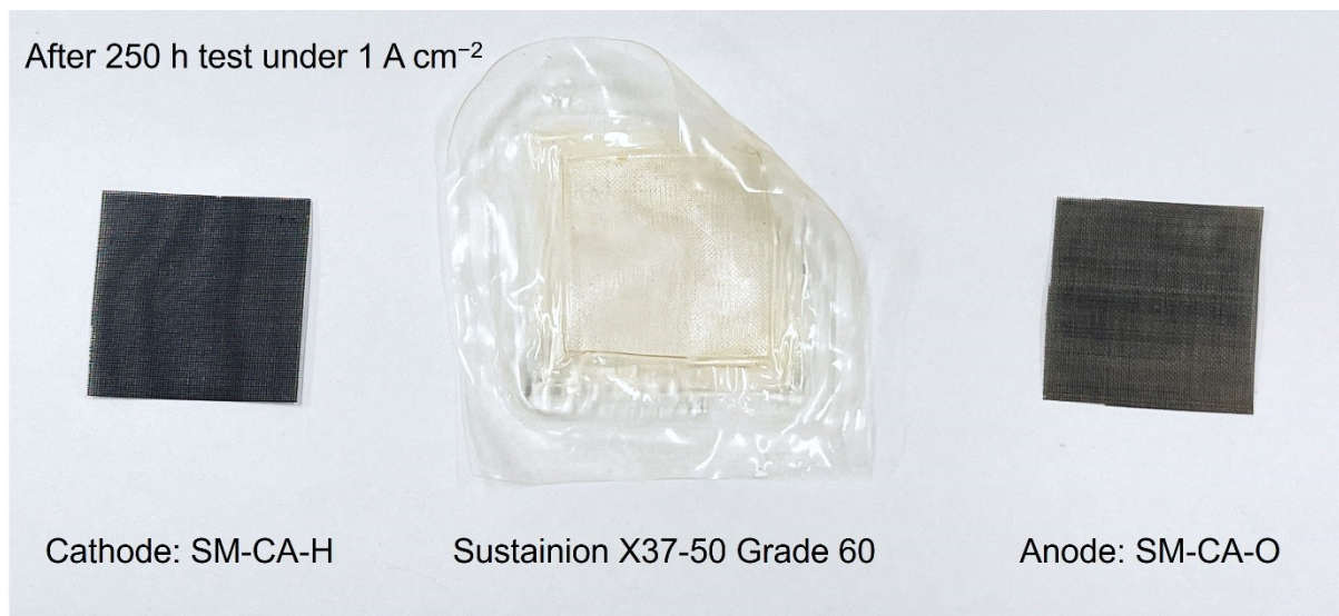
Figure S15. The optical image of the 5 \text{ cm}^2 squared SM-CA-H(-)||SM-CA-O(+) electrodes after 250 h durability test under 1 \text{ A cm}^{-2} .
