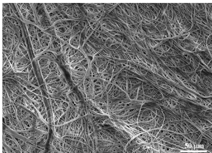
Fig. S5. Typical SEM image of cellulose film.
