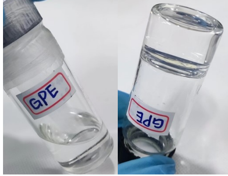
Figure S4 The optical photographs of the precursor solution before (a) and after (b) thermal polymerization.
