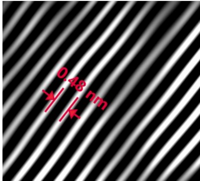
Figure S8. Diffraction fringes obtained by the corresponding inverse Fourier transform in region II.
