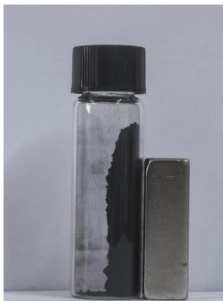
Fig. S2 Photo of a magnet attracting CoNiZnO@NC-30.
