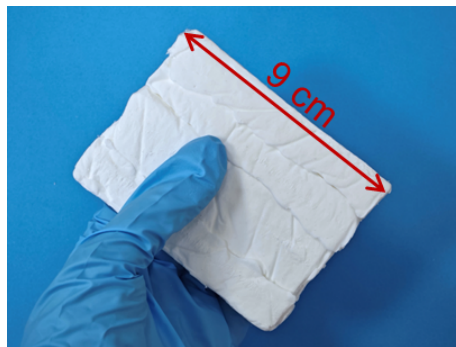
Fig. S12 Digital photo of large-size M10 prepared by a block-by-block freeze-casting method.
