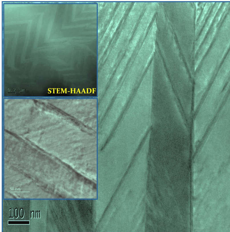
1 Figure S9. Structural domain strain in the herringbone structure. Top inset shows the STEM- 2 HAADF dark field image of highly strained boundaries, and bottom inset shows the 3 magnified view of highly strained domain boundaries.
