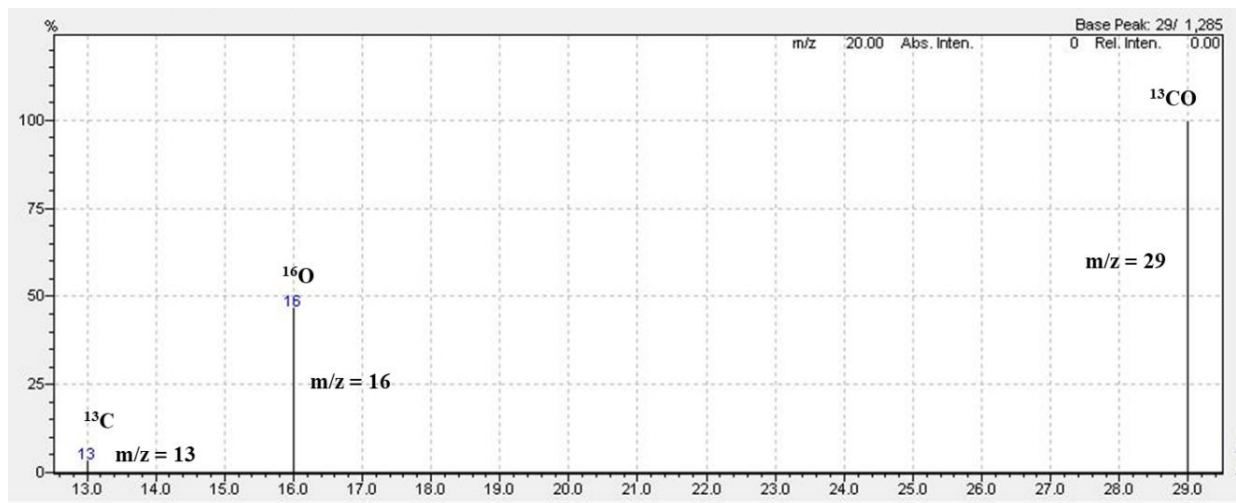
Figure S10: GC-MS analysis using ^{13}\text{CO}_2 as source of \text{CO}_2 after photoreduction reaction.
