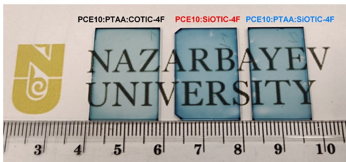
Fig. S1. Photo image of BHJ layers on a neutral paper background.
