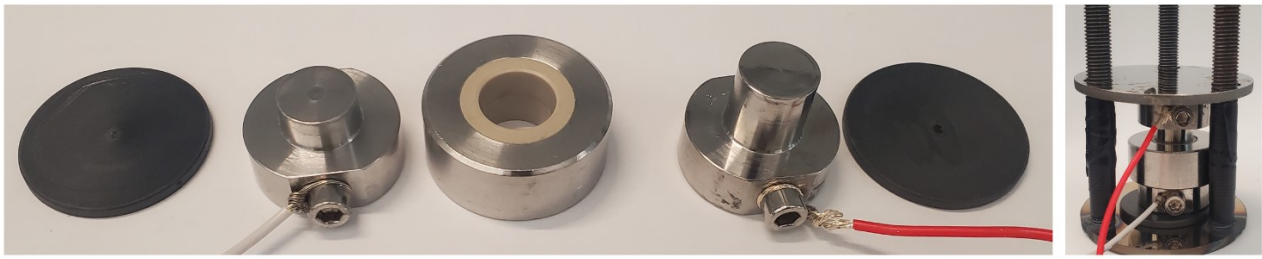
Figure S24. Images of cell components utilized to measure the electronic conductivities of lithium niobate powders, and the assembled cell.
