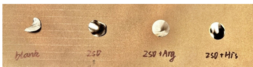
Figure S20 After the flame-retardant test of different electrolytes, the morphology of the glass fiber: (a) normal glass fiber separator, (b) glass fiber separator soaked into baseline electrolyte. (c) glass fiber separator soaked into 0.1M arginine, (d) glass fiber separator soaked into 0.02M histidine.
