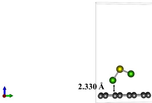
**Figure S7.** Modeling of the structure after the adsorption of Li<sub>2</sub>S on graphene.
