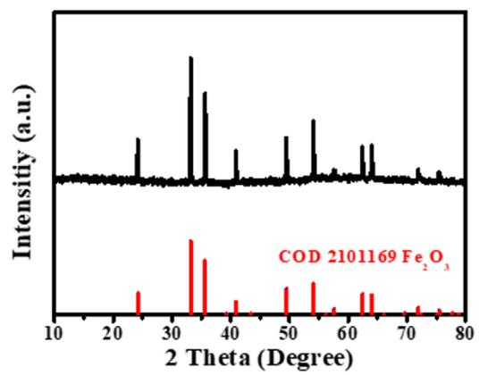
**Fig. S5** XRD pattern of the residue of Fe/N-CNF after TGA analysis.
