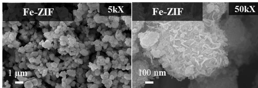
**Fig. S3** SEM images of Fe-ZIF particles.
