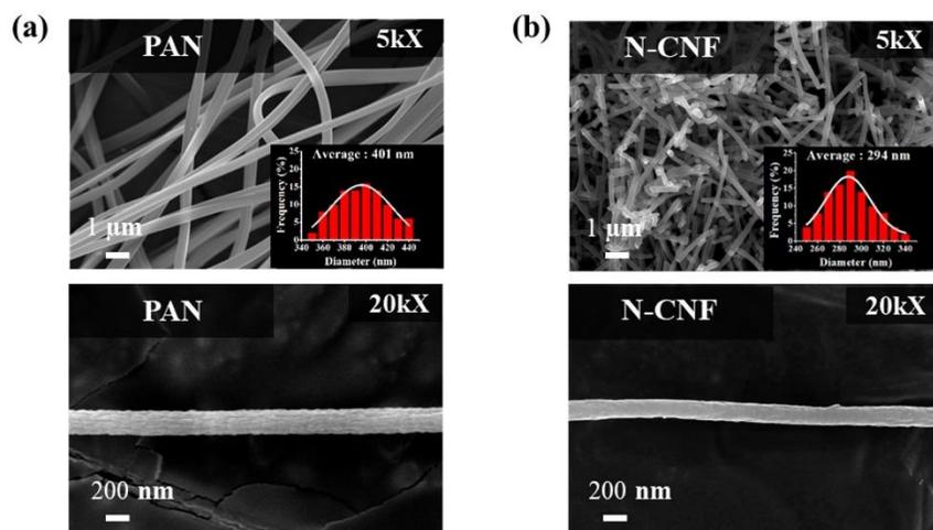
**Fig. S1** SEM images and size distributions of (a) PAN fiber and (b) N-CNF.
