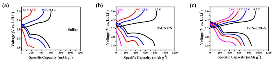
**Fig. S10** Galvanostatic charge and discharge curves of the cells with (a) sulfur, (b) N-CNF and (c) Fe/N-CNF as the cathodes measured at different rates 0.2 to 2.0 C.
