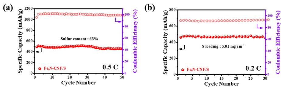
**Fig.S11** Cycle analysis of electrodes with increased (a) sulfur content and (b) sulfur loading for practical application in Li-S batteries (LSBs).
