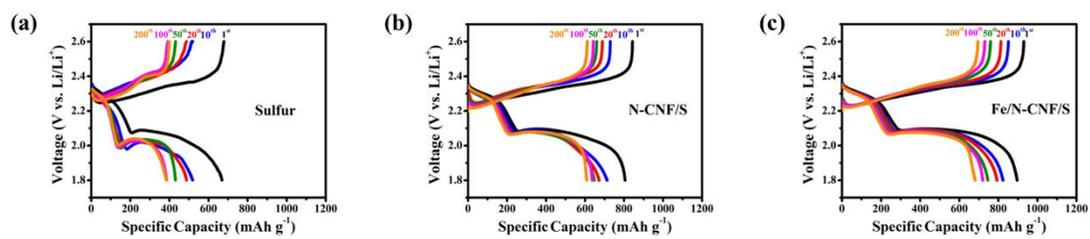
**Fig. S9** Galvanostatic charge and discharge curves of the cells with (a) sulfur, (b) N-CNF and (c) Fe/N-CNF as the cathodes measured at 0.2 C for 1st, 10th, 50th, 100th, and 200th cycles.
