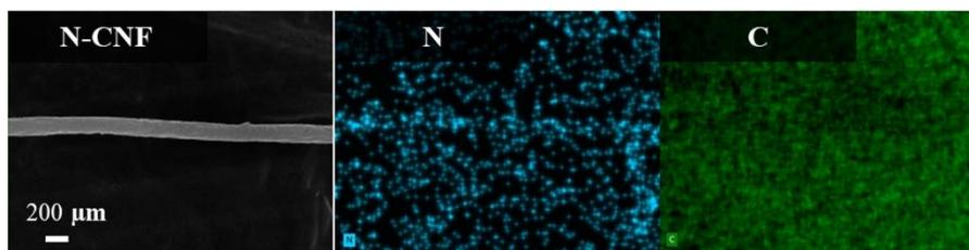
**Fig. S2** EDS mapping images of N-CNF.
