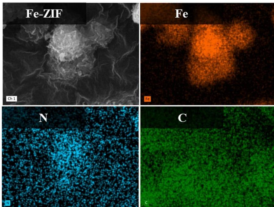
**Fig. S4** EDS mapping images of Fe-ZIF particles.
