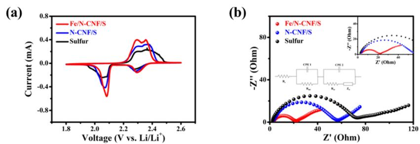
**Fig. S8** (a) CV profiles and (b) Nyquist plots of the cells with Fe/N-CNF, N-CNF, and sulfur as the cathodes after 30 cycles.
