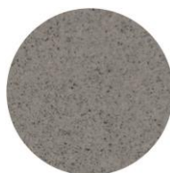
Fig. S28 Picture of the powder of the Mg-Fe system material after four cycles of hydrogenation/dehydrogenation experiments under \sim 50 bar of H 2 /CO 2 gas mixture (0.5 bar of partial CO 2 pressure).
